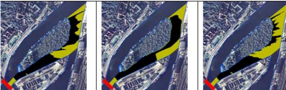
Fig. 10. Results of modified viewshed analysis for TIN, LOD1 and LIDAR DSM [own study]
