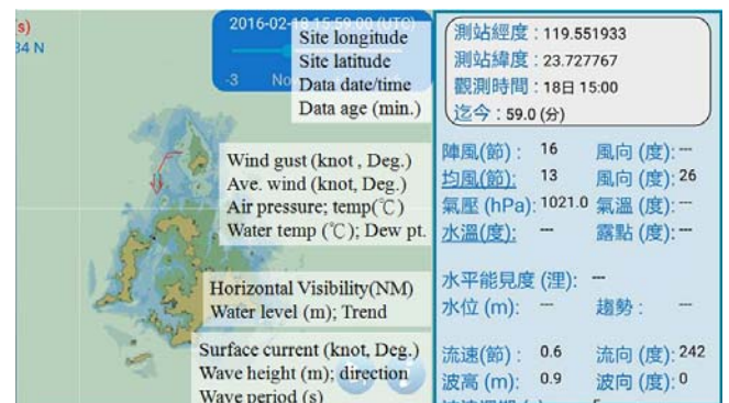
Figure 5. AIS-weather APP with the information panel showing data of the selected buoy site (highlighted in red).
