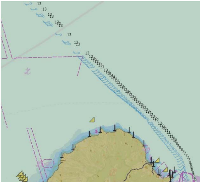
(b) Wind speed reported from a passenger ship Figure 7. Shipboard weather observation reports received at MHCC in CWB.
