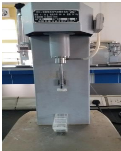
Fig. 2. XFG flotation machine used for the flotation tests
