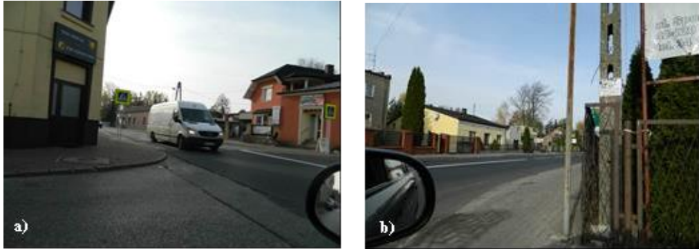
Fig. 4. Limited visibility caused by: a) a building and a road arch, b) a fence and vegetation
