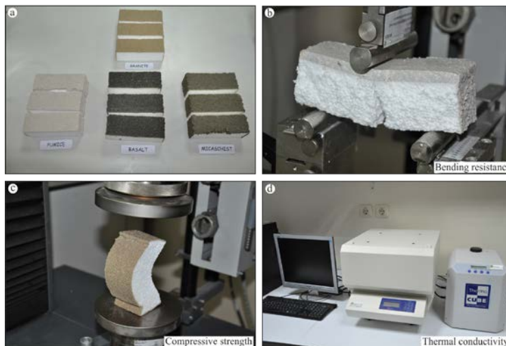
Fig. 2. Thermo-physical tests a) samples b) bending resistance test c) compressive strength test d) thermal conductivity test
