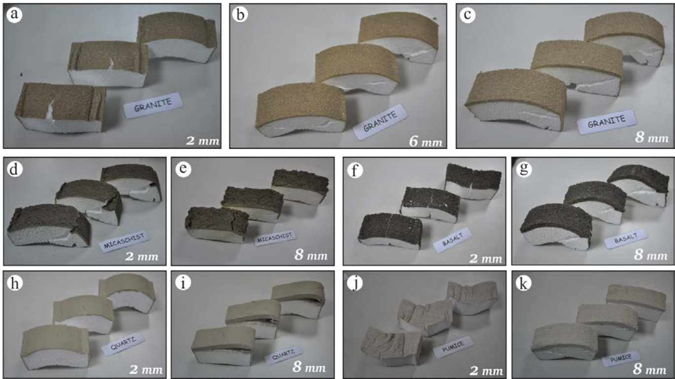
Fig. 3. Deformation styles of the test samples under compressive stress
