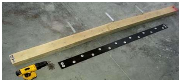
Fig. 1. Softwood beam and CFRP plate
