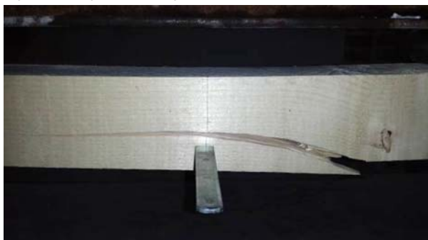
Fig. 11. Typical tensile failure mode of unreinforced beams near a knot or due to grain deviation
