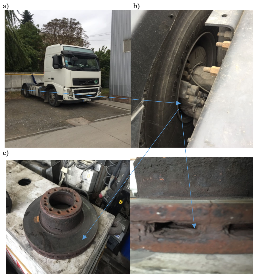
Fig. 1. VOLVO FH 500 truck tractor: a) general view; b) a fragment of the running gear; c) brake disc
