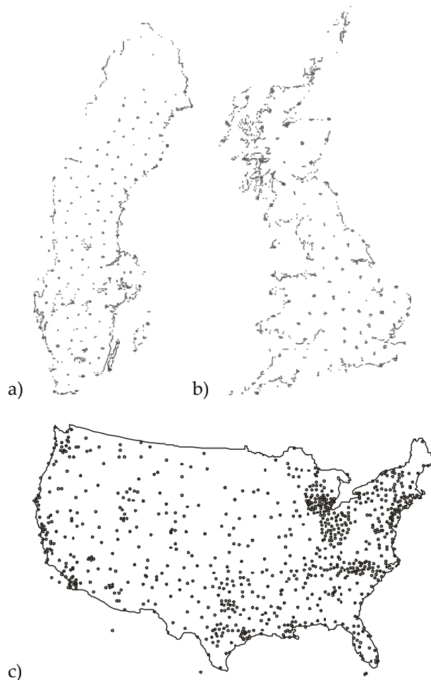
Figure 2. Architecture of selected active geodetic networks: a) SWEPOS – Sweden, b) OS-AGN – Great Britain, and c) CORS – USA
