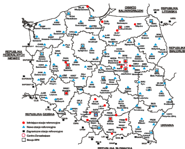
Figure 3. Location of ASG-EUPOS reference station system
