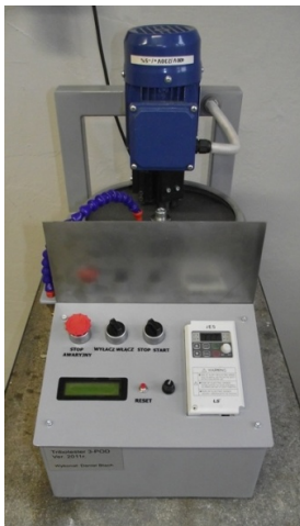
Fig. 2. Scheme of the method used, the specimen and general view of the Tribotester 3-POD apparatus
