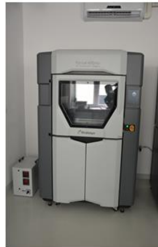
Fig. 4. Stratasys FORTUS 400mc industrial 3D printer [own development]
