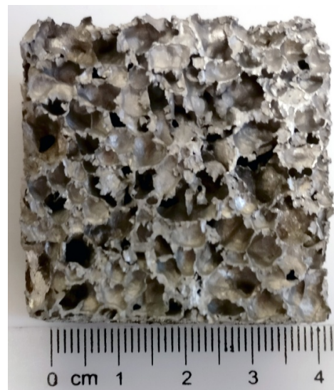
Fig. 1. An example of metal-ceramic foam (values given in centimeters)
