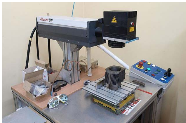
Rys. 2. Laser Nd: YAG Allprint DN ( \lambda = 1064 \text{ nm} , f = 1 \div 100 \text{ kHz} , E = 50 \text{ J} , P = 50 \text{ W} )
