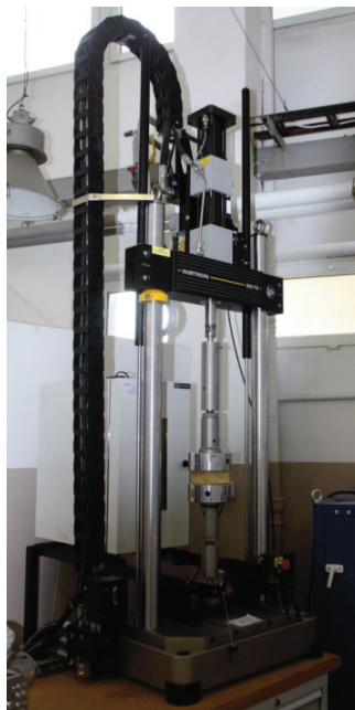
Fig. 1. Static and dynamic testing machine INSTRON 8872
