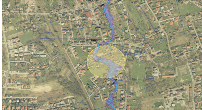
Fig. 8. The danger zone on the river Serafa due to the loss of channel capacity
