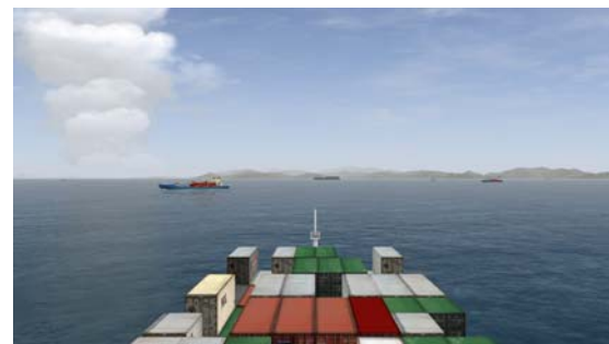
Figure 7. The situation when the bow crossing distance was 1.2 miles as a result of the collision avoidance manoeuvre (Manoeuvring using a simulator)
