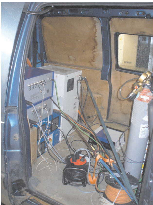
Fig. 3. Measuring equipment (PEMS type) mounted on the vehicle
