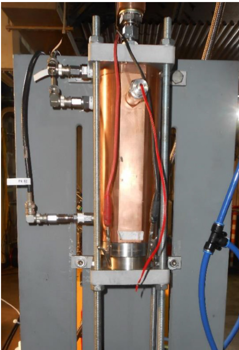
Fig. 2. 100N monopropellant test engine for the nitromethane engine firings
