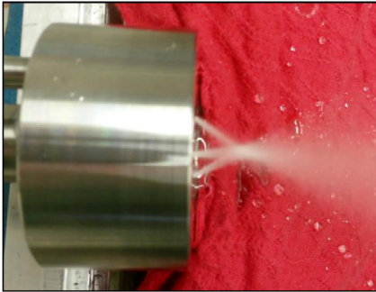
Fig. 4. Fuel elements functional test with water and at ambient condition of the bi-propellant injector head
