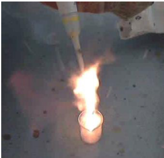
Fig. 3. 'Hypergolic' reaction between hydrogen peroxide and TNO fuel PT28
