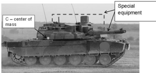
Fig. 6. Arrangement of special equipment in a combat vehicle
