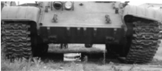
Fig. 9. An example of explosive position under the vehicle in its longitudinal axis
