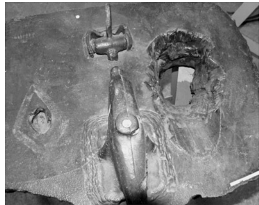
Fig. 4. An armour after missile impact (armour after tests in the Motor Vehicle Institute of the Military Technical University) – a photo from own collections
