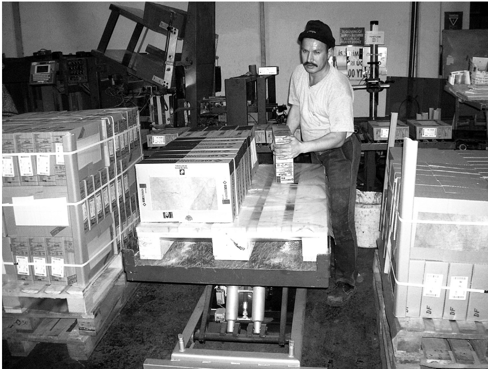
Figure 7. The stacking by pushing boxes onto a pallet.
