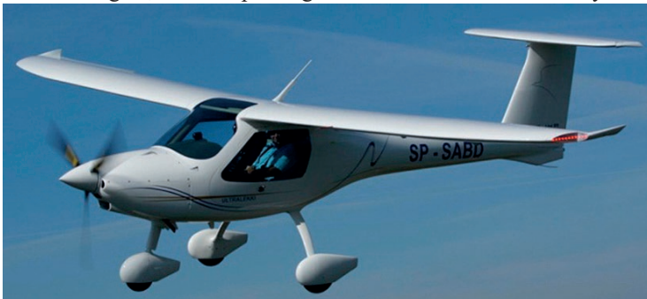
Photo 1. MP-02A Czajka Optionally Piloted Vehicle [courtesy of "Aero-Kros" sp. z o.o. in Krosno]
