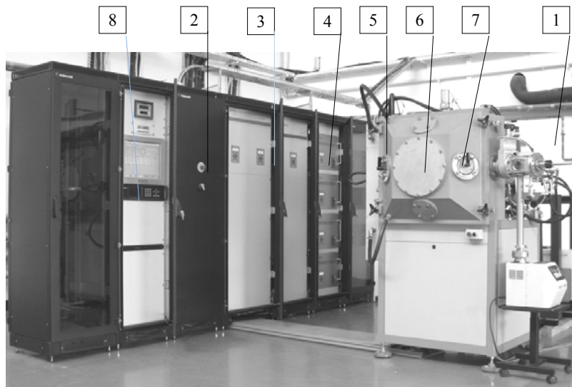
Fig. 2. Specialised test stand: 1 – vacuum chamber with, 2 – control cabinet with a PC and control apparatus, 3 – electrical switchgear module, 4 – bias power supply, 5 – resistance heater power supply, 6 – arc source power supplies, 7 – magnetron source power supplies, 8 – cabinet for additional equipment (instrumentation)
