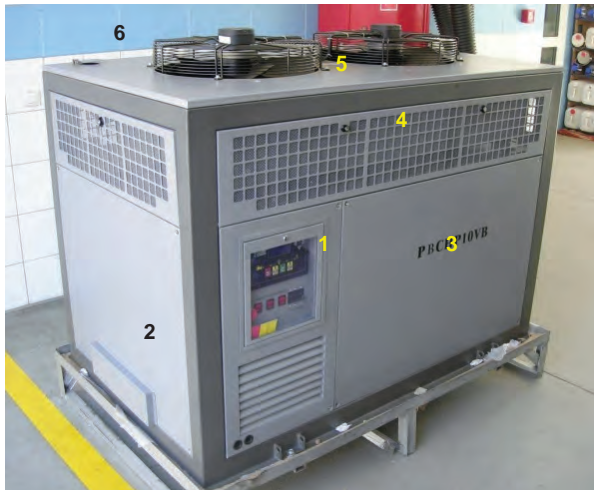
Fig. 1. PBCHP10VB CHP unit: 1 – control panel, 2 – power connection, 3 – main unit chamber with engine, current generator and operating heat exchanger, 4 – upper unit chamber with radiator, equalizing tank, air filter and exhaust silencer, 5 – engine radiator fans, 6 – exhaust gas outlet
