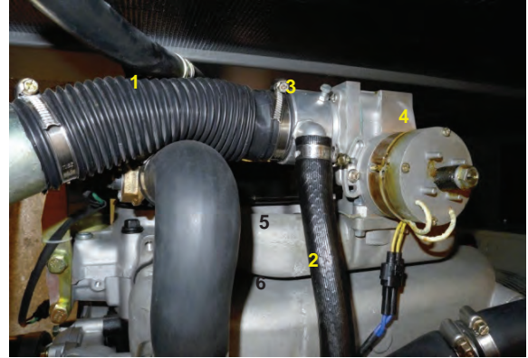
Fig. 4. Gas fuel and air feed system components: 1 – air feed pipe, 2 – conduit feeding gas from the reducer, 3 – gas and air mixer, 4 – electronic throttle valve unit, 5 – suction manifold, 6 – exhaust manifold
