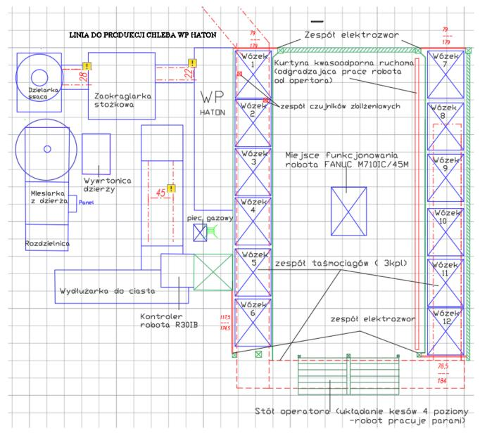
Figure 1 Layout diagram of a robotic production system based on a ROB1 robot with a KON1 controller in bakery X (Source: Own work based on research performed in a bakery)
