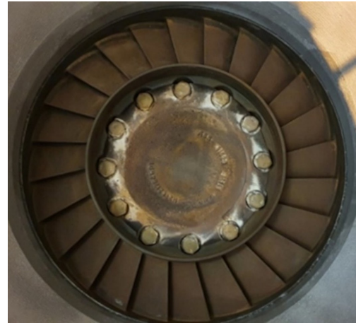
Fig. 2. Blade rim of expansion instruments of a turbocharger of the ABB TPL 67-C type contaminated with deposits of fuel combustion products
