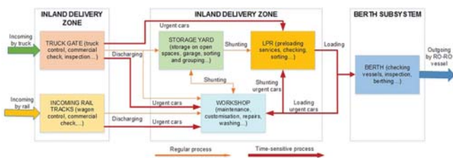
Fig. 4. Workflow of main processes on outbound oriented maritime car terminal
