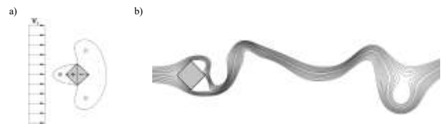
Fig. 2. Influence of the probe cross-section on the streams of fluid assigned numerically [9]: a) averaged in time, b) variable in time for the selected time value
