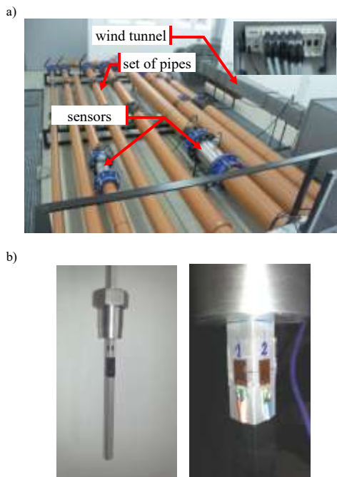
Fig. 6. a) The view of the stand. b) The flow sensor with strain gauges
