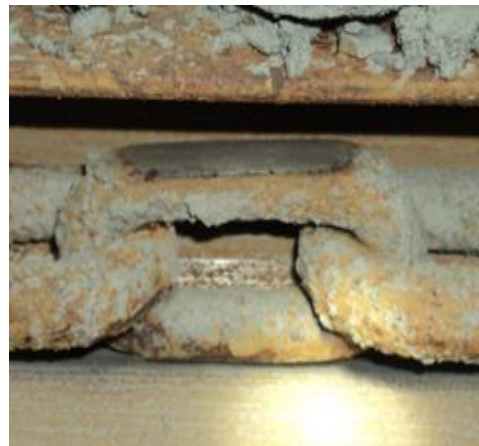
Fig. 8. Link abrasion on the conveyor trough [15]
