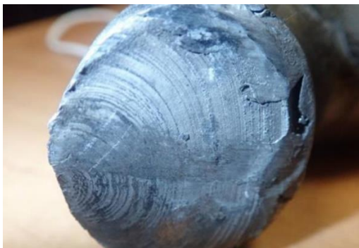
Fig. 12. Fatigue fracture of a chain link [8]
