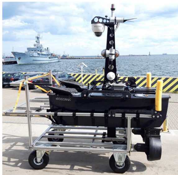
Fig. 3 The Neogobius system in the transport variant.
