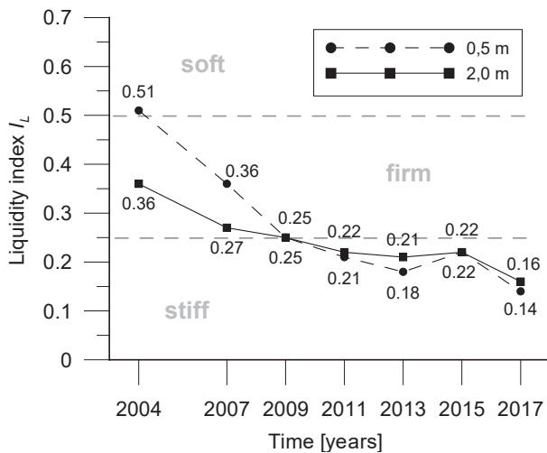
Figure 8: Changes in the retaining embankment soil liquidity index (mean values from three boreholes).
