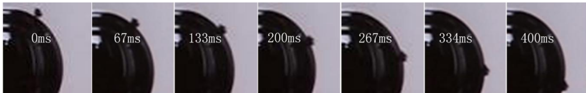
Fig. 11. Motion of an irregular hematite floc on the bubble surface
