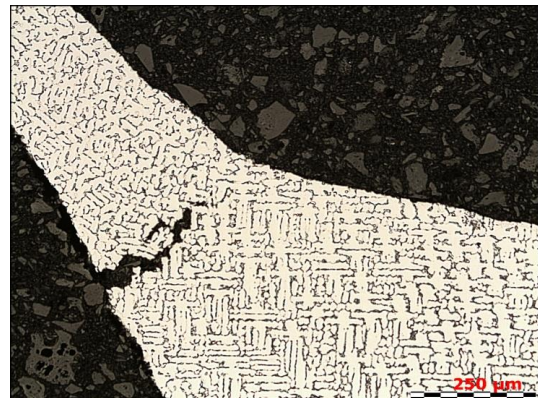
Fig. 4. Microstructure of the Co-Cr-Mo alloy with a visible casting defect – intercrystalline crack: a) magnification 50x, b) magnification 100x
