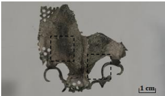
Fig. 1. Cast of a frame bracket prosthesis with a visible casting defect in the form of blisters
