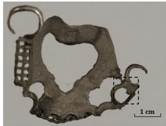
Fig. 3. Frame prosthesis with a visible cold fracture on the side of the bracket
