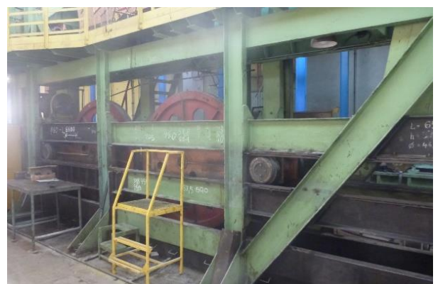
Fig. 4 View of the P4-GIG-2 fatigue testing machine
