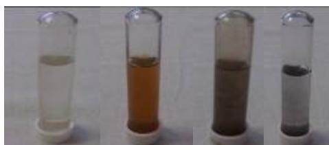
Figure 1. Images of water dispersions of silver particles prepared by reduction of \text{Ag}^+ in ammonia. From left: dispersions – ion silver; nano-particles of silver with the size approx. 25 to 50 nm.
