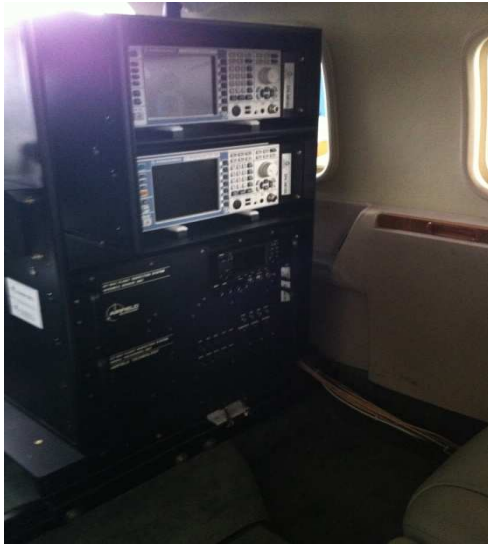
Fig. 2. Airborne and ground equipment AT-940 with spectral analyzer and selective millivolt meter.
