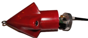
Fig. 2. Acoustic warhead of the CZT measuring unit with the analysis, recording and data transmission module
