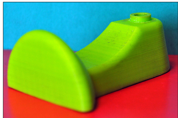
Fig. 3. Element made in FDM method
