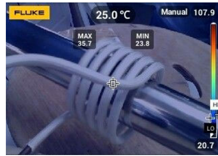
Fig. 13 Experimental stainless steel pipe and induction coil at room temperature
