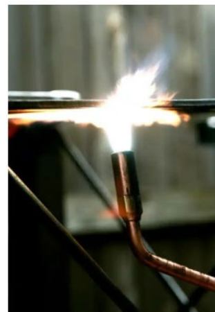
Fig. 1. The use of gas fire to heat the surface of the workpiece
