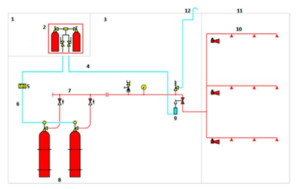
Figure 4. Diagram of gas fire-extinguishing system (CO<sub>2</sub>): 1 – control station, 2 –release cabinet, 3 – CO<sub>2</sub> cylinder compartment, 4 – release line – distribution valve, 5 – time delay unit, 6 – release line – cylinders, 7 – manifold, 8 – CO<sub>2</sub> cylinder bank, 9 – distribution valve, 10 – distribution pipelines with nozzles, 11 – protected space, 12 – to free air (Wilhelmsen Technical Solution, 2014)
