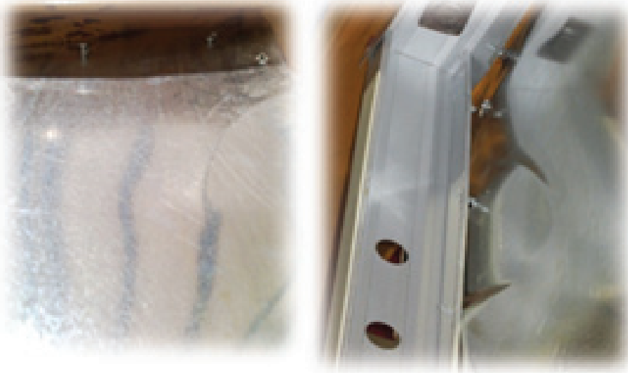
Figure 5. Failure modes of specimens type I a. Rivet tilting and hole bearing; b. Screw pull-out
