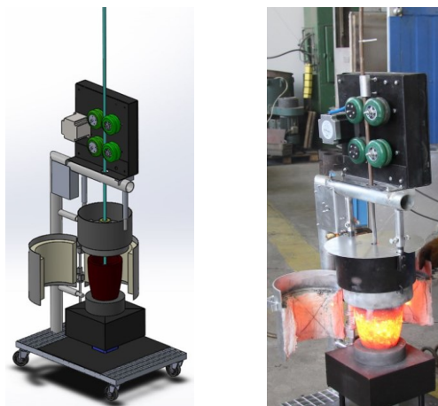
Fig. 1. Laboratory set-up for cast iron spheroidisation by means of the PE method
