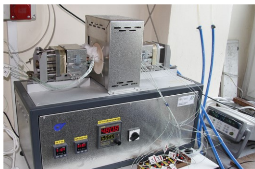
Fig. 10. Research set-up for testing the thermal conductivity of materials, including foundry metals and alloys
