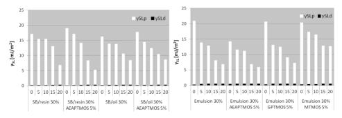
Fig. 5. Values of  $\gamma_{SL}$  and its components in the function of the number of aging cycles (0–5–10–15–20) for wood surface treated with selected systems
