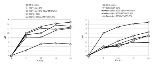
Fig. 6. Fluctuations in  $\Delta E$  in the function of the number of aging cycles for wood surfaces treated with selected systems
