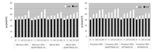
Fig. 3. Values of  $\gamma_s$  and its components in the function of the number of aging cycles (0–5–10–15–20) for wood surface treated with selected systems
