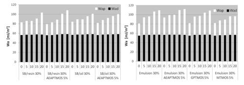
Fig. 4. Values of  $W_a$  and its components in the function of the number of aging cycles (0–5–10–15–20) for wood surface treated with selected systems
