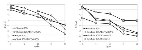
Fig. 2. Values of angle  $\Theta$  in the function of the number of aging cycles for wood surface treated with selected systems
