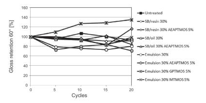
Fig. 7. Changes in gloss retention in the function of the number of aging cycles for wood surfaces treated with selected systems
