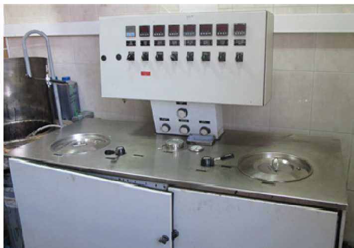
Fig. 1. Lab bitumen emulsion plant SEP-0,3R of Danish company DenimoTech
