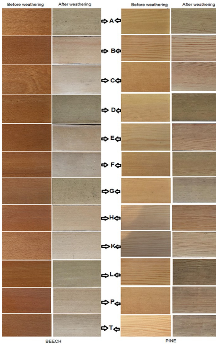
Fig. 4. Wood surfaces treated with acrylic-based coating systems
