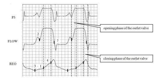
Fig. 3. Signals during VAD's working cycle and position of characteristic points.
