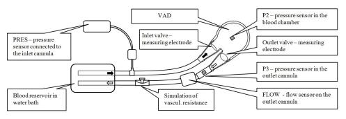
Fig. 1. Flow test stand.
