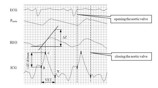
Fig. 2. Physiological signals during a single cardiac cycle and the method of determining the actual impedance change.
