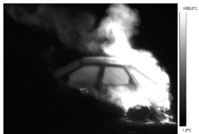
Fig. 2. Thermal image of the car with the measurement point marked
