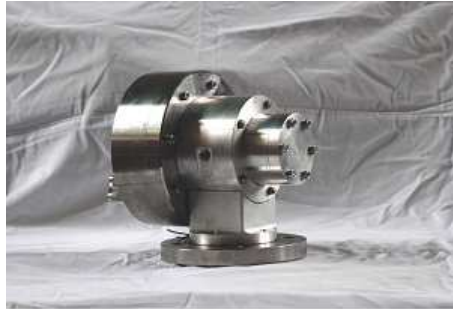
Figure 3: View of vapour ORC microturbine.
