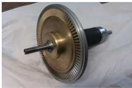
Figure 4: Turbine rotor disk with generator rotor.
