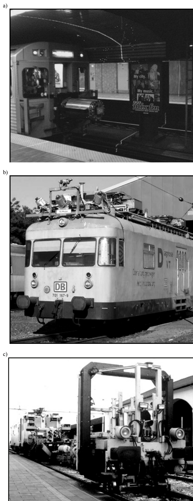
Fig. 5. Gauge surveying systems: a) Balfour Beatty Rail system [23], b) RailMapper [22], c) LIMEZ II [17]
