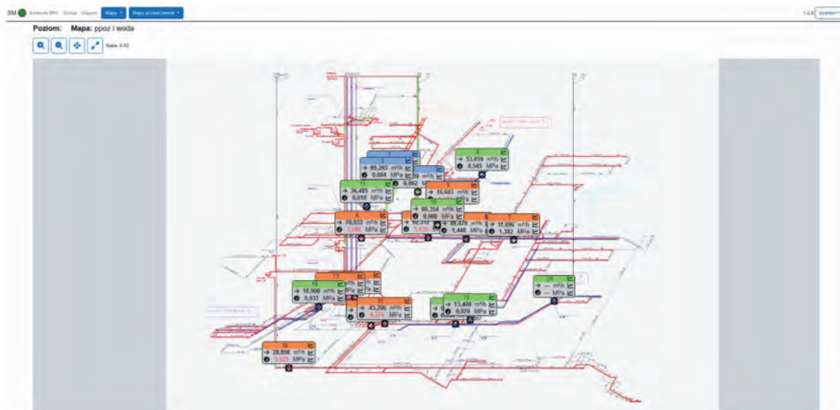
Fig. 3. View of the main synoptic screen of the visualisation application of the SYSMON system with the total indications from the flowmeters at Piast-Ziemowit Hard Coal Mine, Ziemowit Operation
