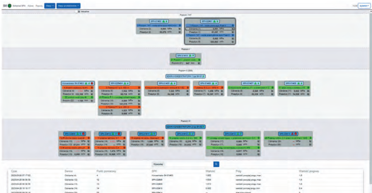
Fig. 2. View of the main synoptic screen of the SYSMON system visualisation application with current indications from the measurement devices at the Piast-Ziemowit Hard Coal Mine, Ziemowit Operation
