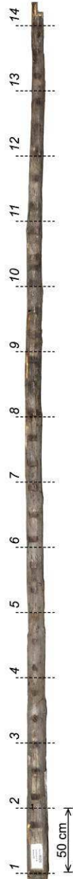
Sample element with indication of points at which the cross-section was measured (view from top)
