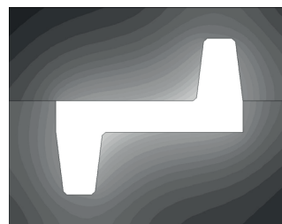
Fig. 16. Temperature field in the mold after 60 s (case B). Maximum value (759 K) is marked in light gray, while minimum value (533 K) is marked in black
